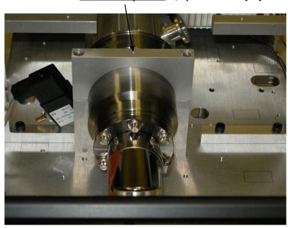
e. Release 6 12-pts bolts with ¼" 12-pts wrench. The bottom bolt can be turned step by step. After release bolts first, then rotate the TP to pull out the bolts completely.
